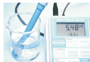
Figure 1: pH can be measured using a pH meter like this one.
