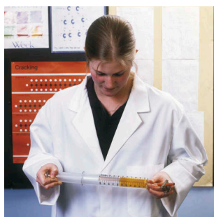
Figure 1b: When pressure is applied the colour changes because the equilibrium shifts in favour of \text{N}_2\text{O}_{4(l)} .
