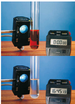
Figure 1: Using a colorimeter to measure a colour change. In clock reactions, there is often a sudden, clear colour change, so a colorimeter isn't always needed.
