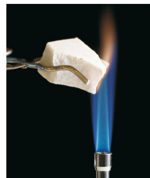
Figure 1: Calcium carbonate ( \text{CaCO}_3 ) being heated to produce \text{CaO} and \text{CO}_2 .
