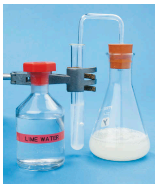
Figure 4: Testing for carbonate ions with hydrochloric acid and limewater.
