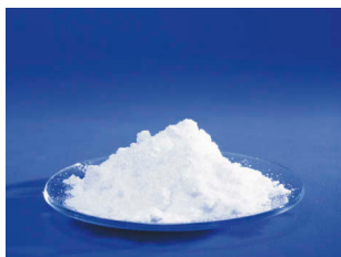
Figure 4: \text{NaBH}_4 powder. This is dissolved in water with methanol to produce a commonly used reducing agent.
