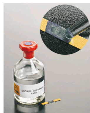
Figure 3: Sodium hydroxide turns this universal indicator paper dark blue, which shows it has a high pH.
