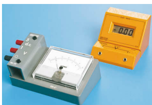
Figure 2: Analogue or digital voltmeters can be used to measure electrode potentials.
