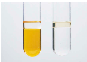
Figure 5: Bromine water turns colourless when shaken with alkenes.
