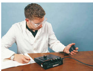
Figure 3: A student using a colorimeter as part of a colorimetry experiment. A digital display shows the absorbance value of a sample at any given moment.
