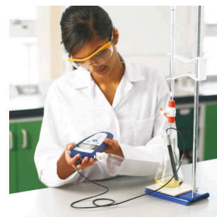
Figure 2: A student using a pH meter to measure pH during an acid–base titration.
