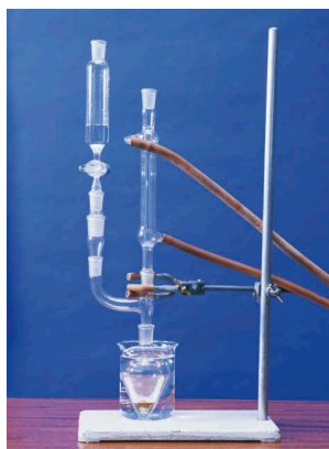
Figure 5: The reflux equipment used to make phenylamine.
