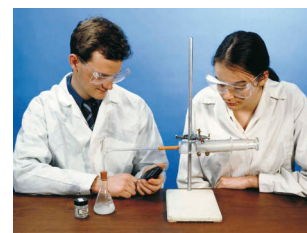
Figure 1: Students measuring the rate of a reaction which produces a gas as a product.
