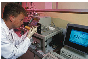
Figure 3: GC-MS being used in a police lab to analyse evidence found at a crime scene.
