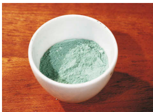
Figure 4: Copper(II) carbonate. A green-blue precipitate is formed when carbonate ions react with aqueous copper(II) ions.
