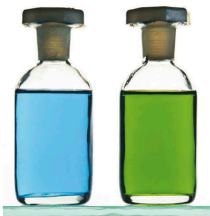
Figure 3: A solution of [\text{Cu}(\text{H}_2\text{O})_6]^{2+} (left). Upon addition of an excess of \text{HCl} , the [\text{CuCl}_4]^{2-} complex forms which turns the solution green (right).
