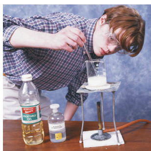
Figure 5: Student making soap by heating vegetable oil with sodium hydroxide.
