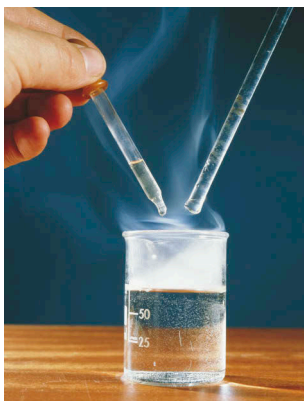
Figure 1: The reaction of an acyl chloride with water. You can see the misty fumes of HCl that are being given off.
