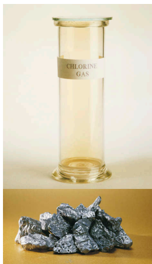
Figure 3: Chlorine (top) has lower melting and boiling points than silicon (bottom). So chlorine is a gas at r.t.p., whilst silicon is a solid.
