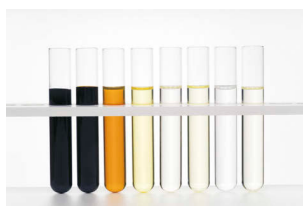
Figure 2: Fractions produced from fractional distillation of crude oil. The fractions are arranged in order of boiling point, with higher boiling points towards the left.
