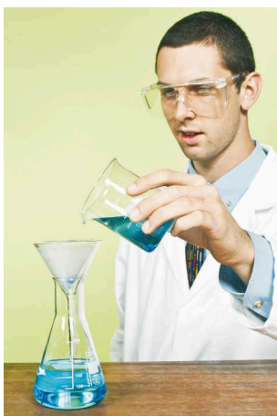
Figure 1: A student pouring and filtering a solution. Some chemicals will be left on the glassware and some will be left on the filter paper.
