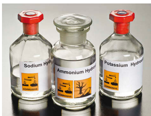
Figure 2: Hazard symbols on bottles of chemicals can tell you if a chemical is dangerous, for example if it is flammable or toxic.
