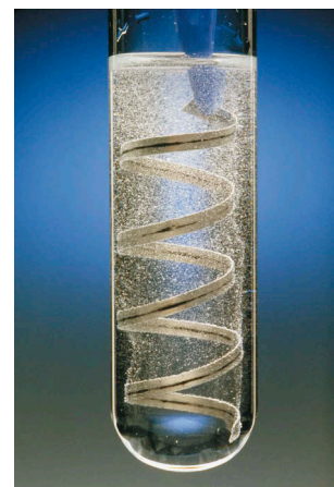
Figure 7: Magnesium ribbon reacting with hydrochloric acid.
