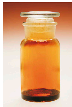
Figure 2: Bromine liquid changing state to become a gas and diffusing to fill the container.
